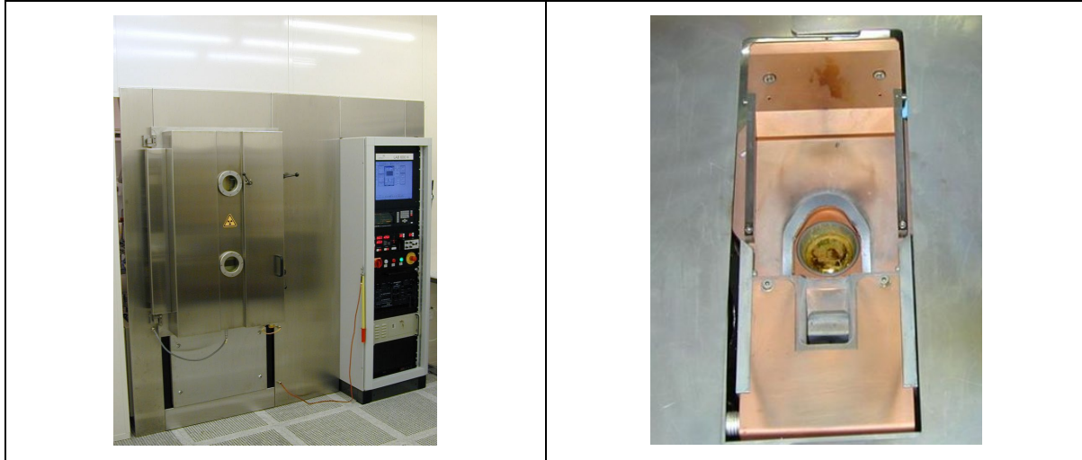
Figure 4. Left: Lab600 evaporator. Middle: e-beam evaporation source. The material is placed in the circular crucible in the middle and heated using an electron beam. Right: boat for evaporation via Joule heating.
